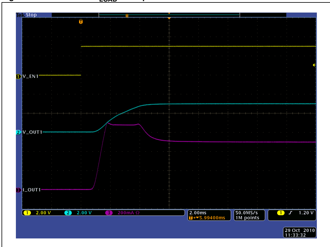
Figure 5. Turn-on for C_{LOAD} = 470 \mu F
