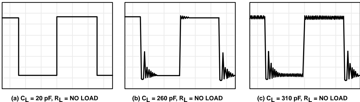
Figure 112. Effect of Capacitive Loads in Low-Bias Mode
