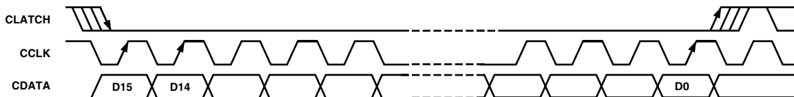
Figure 1. Format of SPI Signal
