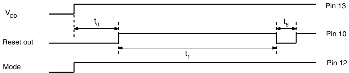
Figure 4-2. Power-up Reset and Mode Switchover
