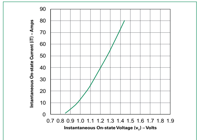
Figure 4: On-State Current vs. On-State Voltage (Typical)
