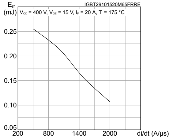
Figure 25. Reverse recovery energy vs diode current slope
