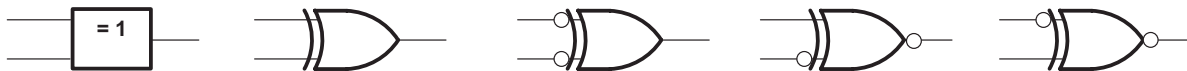
A. These are five equivalent exclusive-OR symbols valid for an 'LV86A gate in positive logic; negation can be shown at any two ports.
