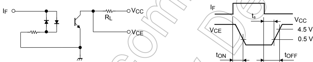
Fig. 1 Switching time test circuit
