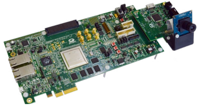
MIPI CSI-2 or Parallel Sensor FMC daughter card options (AR330 Image Sensor Board included)
