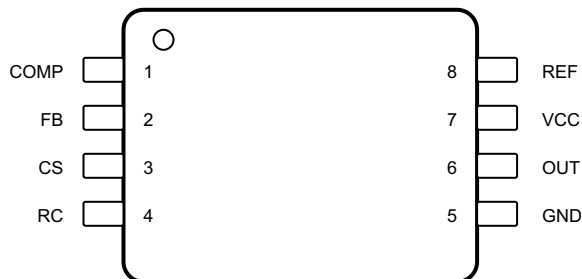
UCC280x and UCC380x PW Package 8-Pin TSSOP Top View
