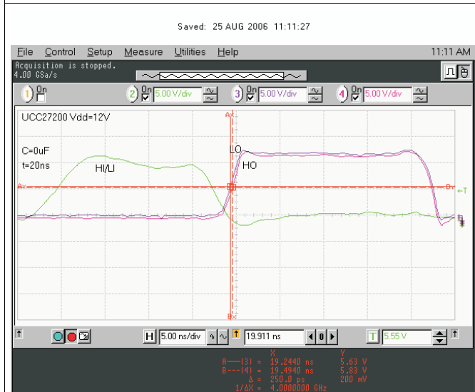
Figure 32. 20-ns Input Pulse Delay Matching
