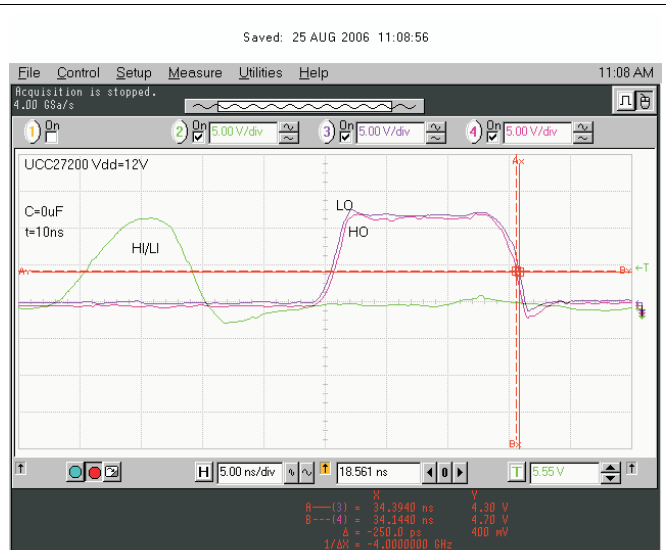
Figure 33. 10-ns Input Pulse Delay Matching
