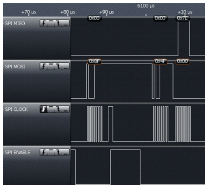
Figure 6-25. Reset FIFO and Read RSSI
