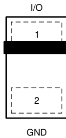
Figure 5-1. DPY Package 2-Pin X1SON Top View
