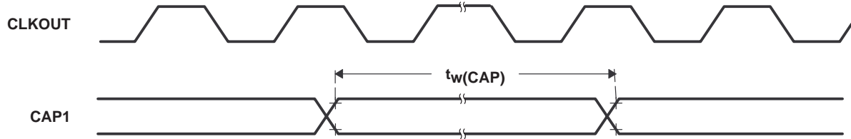
Figure 35. Capture Input Timing
