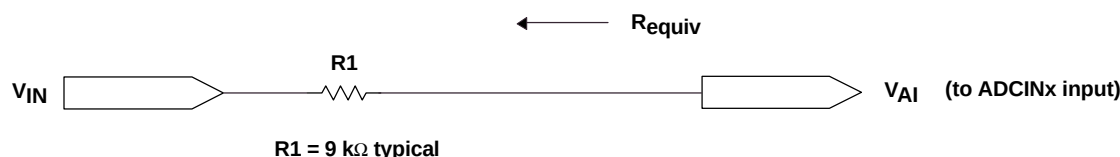
Figure 48. Typical ADC Input Pin Circuit
