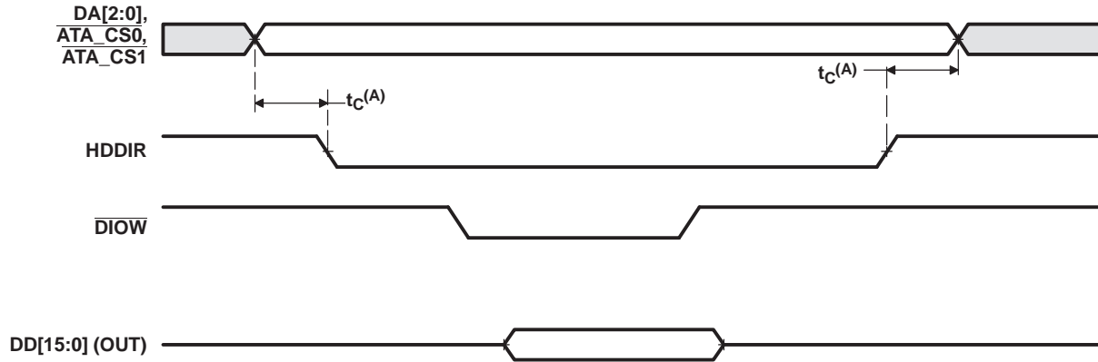
Figure 6-38. ATA/CF HDDIR Taskfile Write/Single PIO Write Timing
