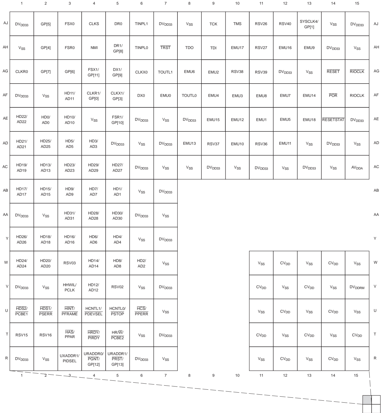
Figure 2-2. C6455 Pin Map (Bottom View) [Quadrant A]
