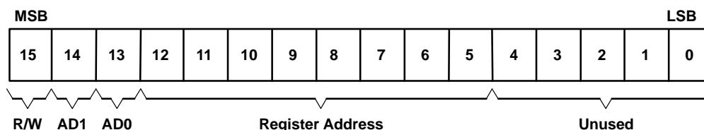
Figure 5. Bit Assignment and Definition for Slot-0 Word
