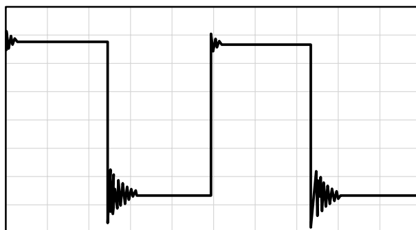
(b) C_L = 130 \text{ pF} , R_L = \text{NO LOAD}
