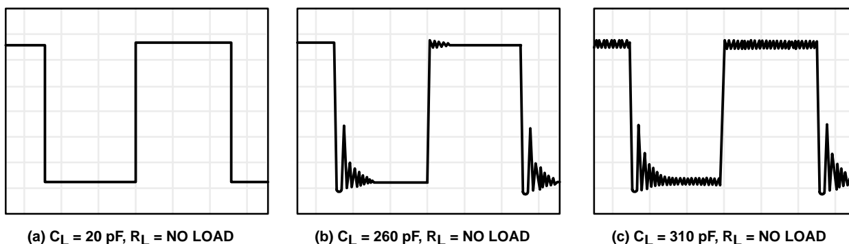
Figure 112. Effect of Capacitive Loads in Low-Bias Mode
