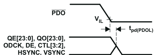
Figure 8-8. Delay From \overline{PDO} Low to Hi-Z Outputs
