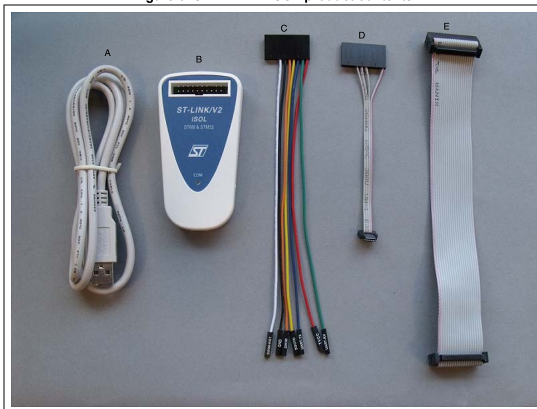
Figure 3. ST-LINK/V2-ISOL product contents
