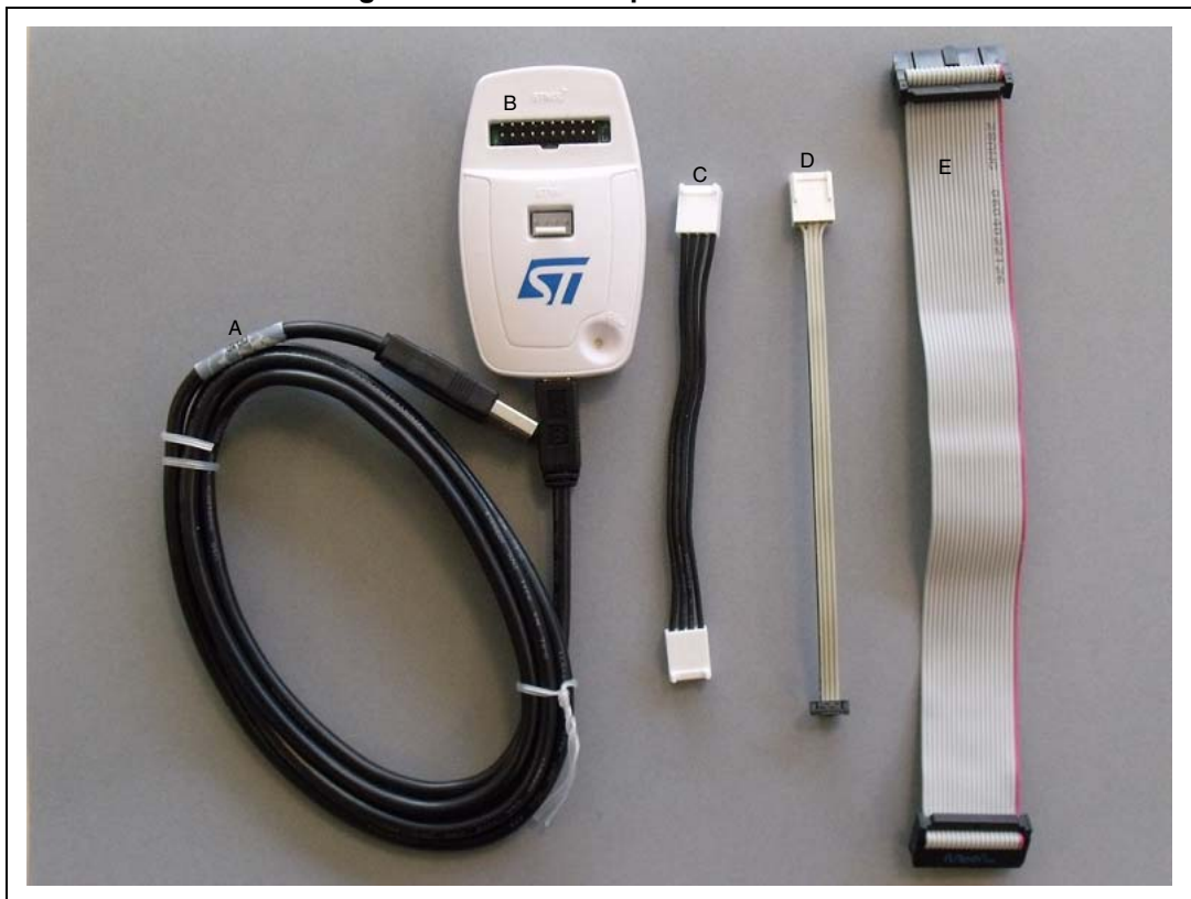
Figure 2. ST-LINK/V2 product contents
