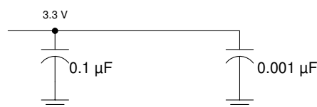
Figure 9-2. Recommended LVDS Bypass Capacitor Layout
