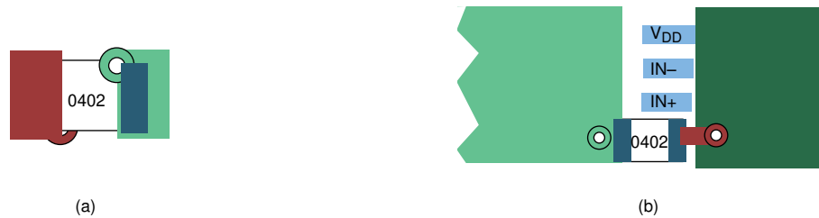
Figure 11-7. Typical Decoupling Capacitor Layouts
