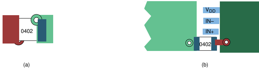
Figure 11-7. Typical Decoupling Capacitor Layouts
