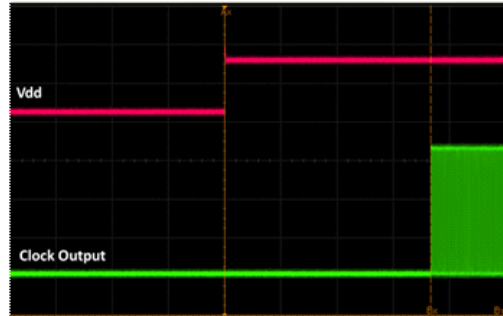
Figure 17. Startup Waveform vs. Vdd
