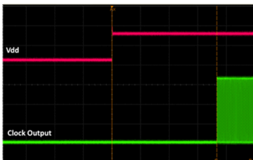
Figure 18. Startup Waveform vs. Vdd
