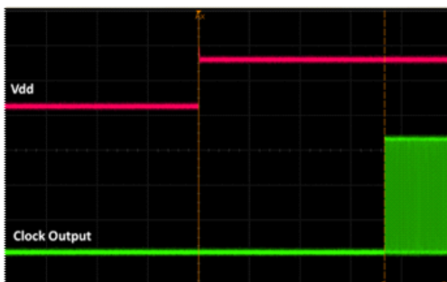
Figure 18. Startup Waveform vs. Vdd
