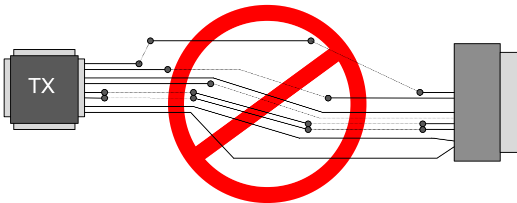
Figure 23. Example of Incorrect Differential Signal Routing
