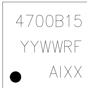
Figure 10. Si4700-B15-GM Top Mark
