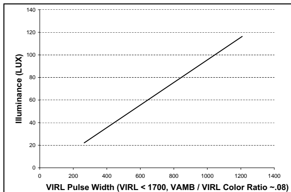
Figure 11. Low Light Transfer Function
