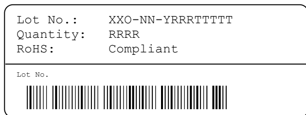
Figure 20: First label on reel: XX = Sensor Type (25 for SHT25), O = Output mode (D = Digital), NN = product revision no., Y = last digit of year, RRR = number of sensors on reel divided by 10 (200 for 2000 units), TTTTT = Traceability Code.
