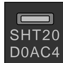
Figure 21 Laser marking on SHT20. For details see text.
