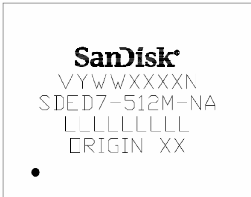
Figure 39: Example of SDED7-512M-NA Product Marking
