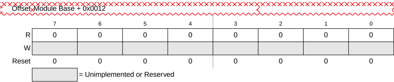
Figure 13-24. Flash Reserved6 Register (FRSV6)
