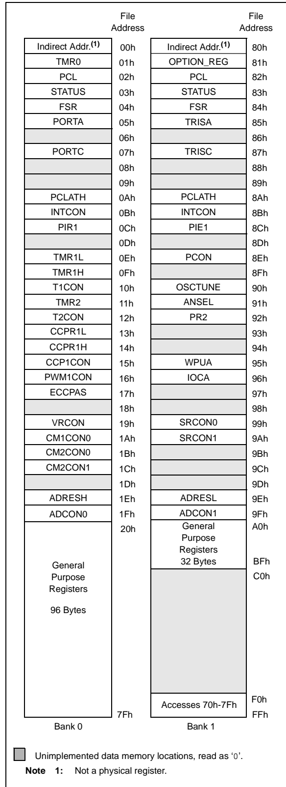
FIGURE 2-4: DATA MEMORY MAP OF THE PIC16F616/16HV616
