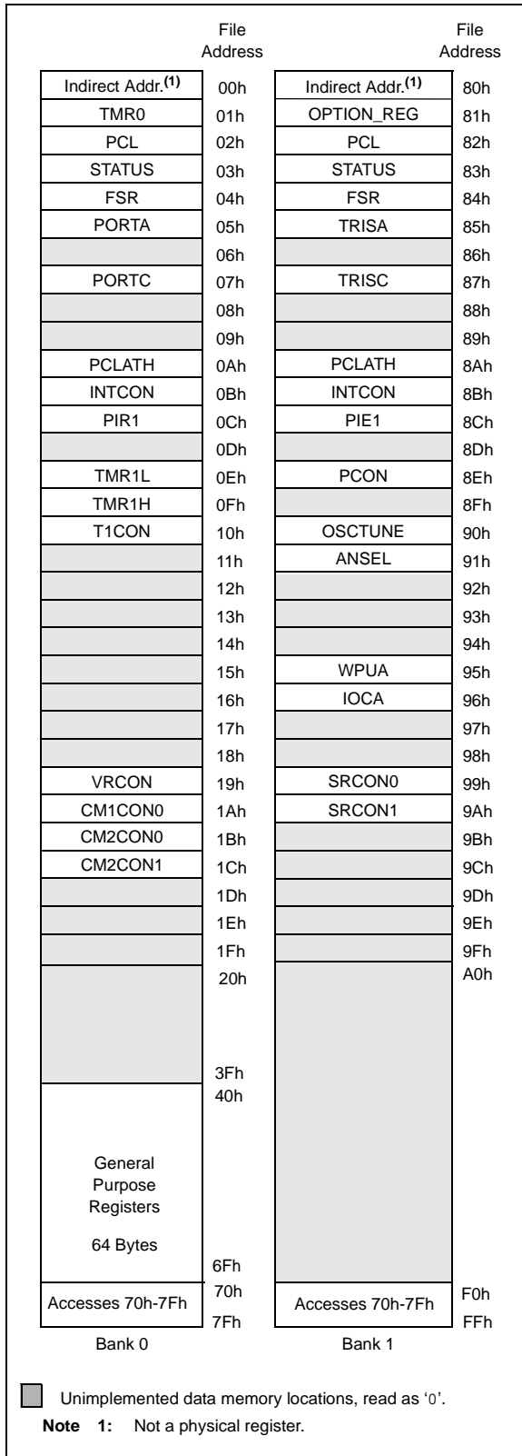
FIGURE 2-3: DATA MEMORY MAP OF THE PIC16F610/16HV610
