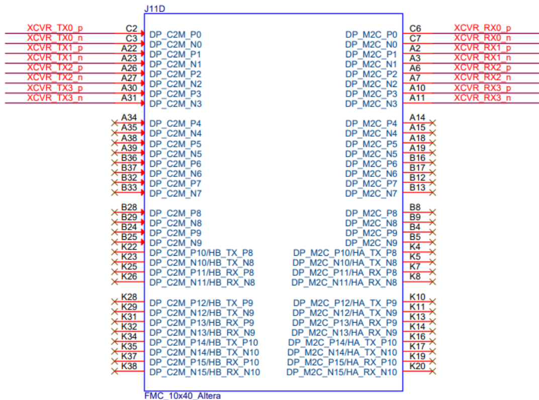
Figure 3-1 Signal names of XTS-FMC connector part 1
