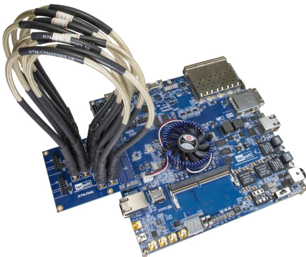
Figure 4-6 The Connections between the XTS-FMC and HAN Pilot Platform board
