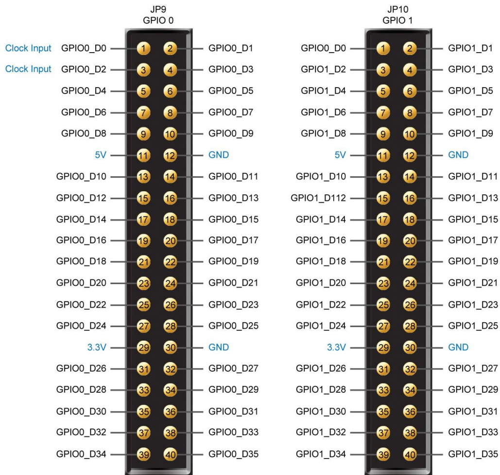
Figure 2-21 Pin Distribution of the GPIO Expansion Headers
