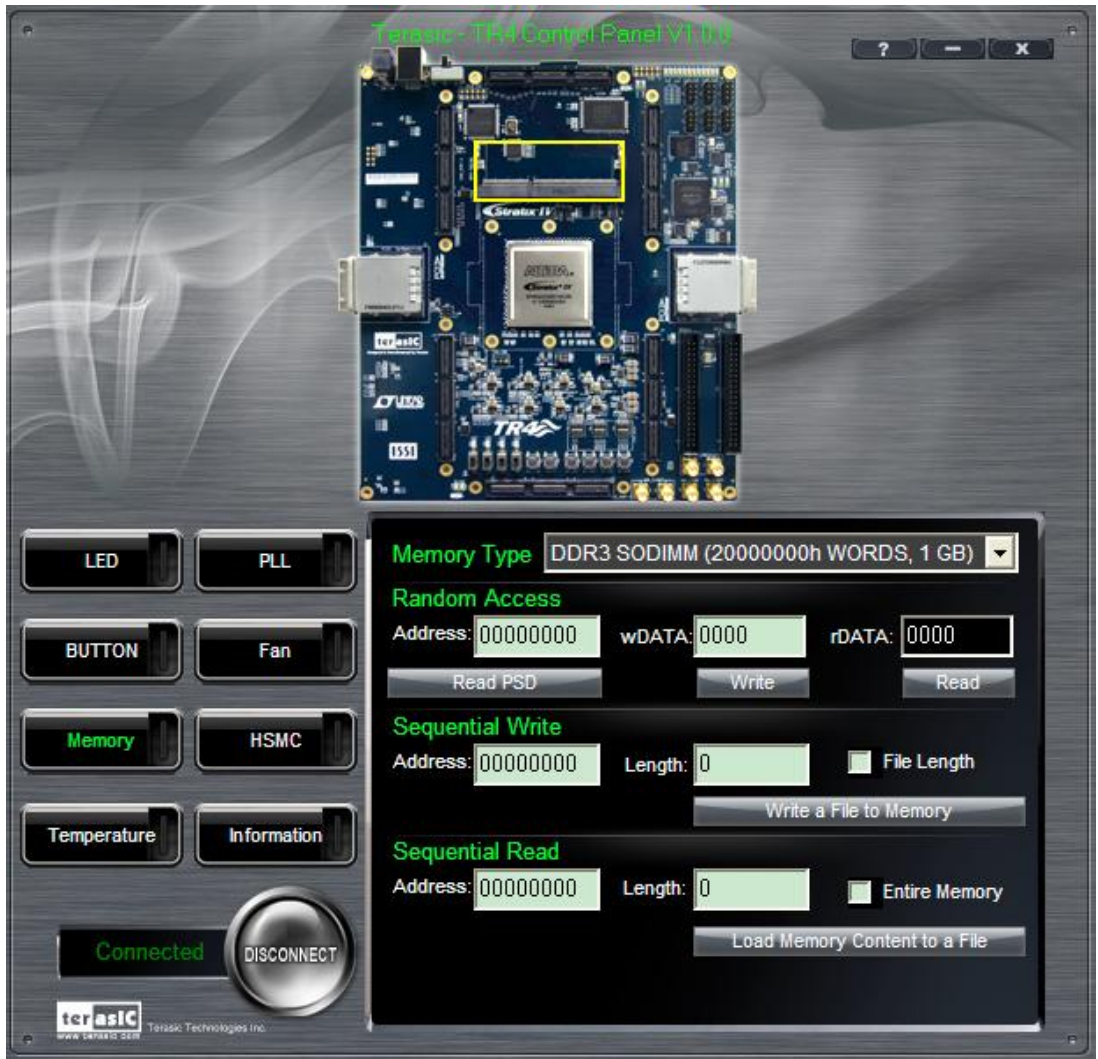
Figure 3-7 Access DDR3 SO-DIMM Memory
