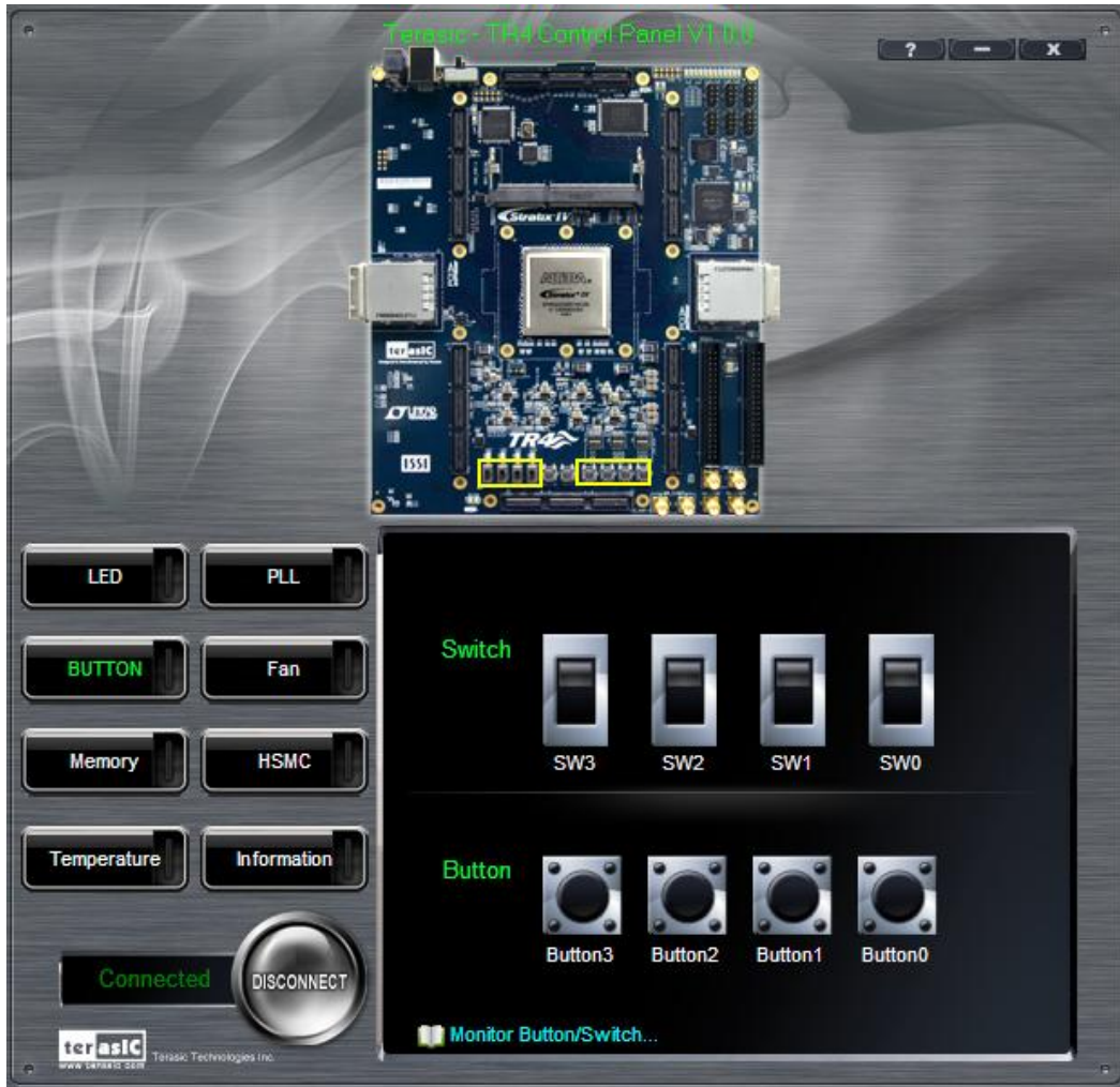
Figure 3-6 Monitoring Switches and Buttons
