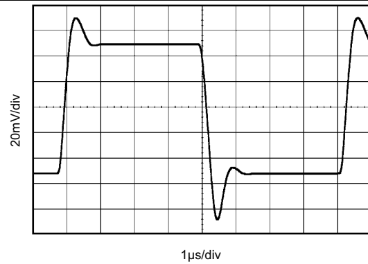
Figure 20. Large-Signal Step Response G = 1 , C_L = 1500\text{ pF} , V_S = \pm 15\text{ V}
