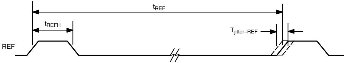
Figure 5. REF Input Timing Diagram
