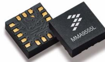
16-pin LGA 3 mm x 3 mm x 1 mm Case 2094-01
