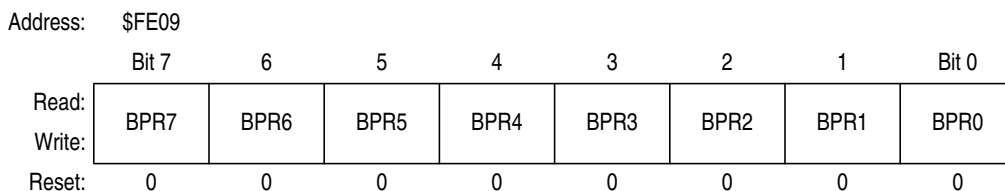
Figure 2-5. FLASH Block Protect Register (FLBPR)
