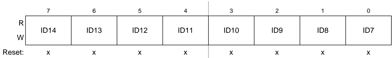
Figure 11-28. Identifier Register 2 (IDR2) — Extended Identifier Mapping
