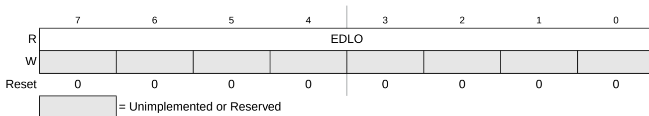
Figure 4-16. EEPROM Data Low Register (EDATALO)
