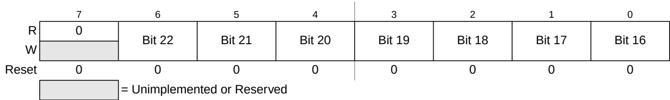
Figure 20-15. Debug Comparator Address High Register (DBGXAH)
