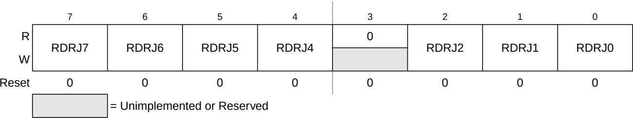
Figure 23-59. Port J Reduced Drive Register (RDRJ)
