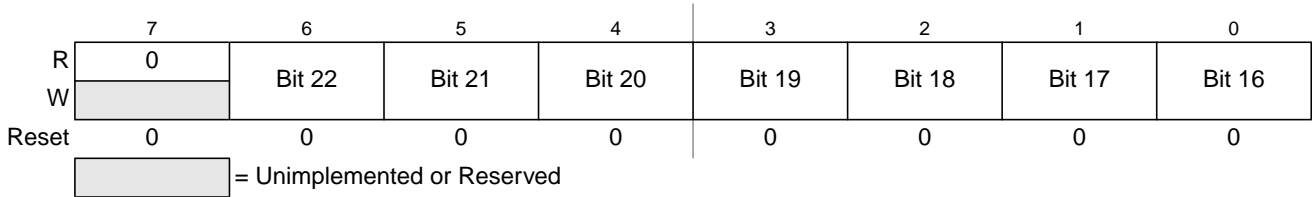
Figure 20-15. Debug Comparator Address High Register (DBGXAH)
