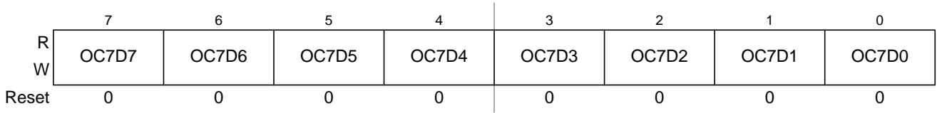
Figure 7-6. Output Compare 7 Data Register (OC7D)
