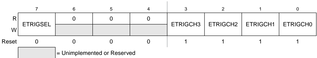
Figure 4-4. ATD Control Register 1 (ATDCTL1)
