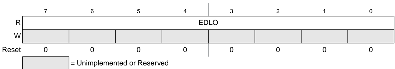
Figure 26-16. EEPROM Data Low Register (EDATALO)
