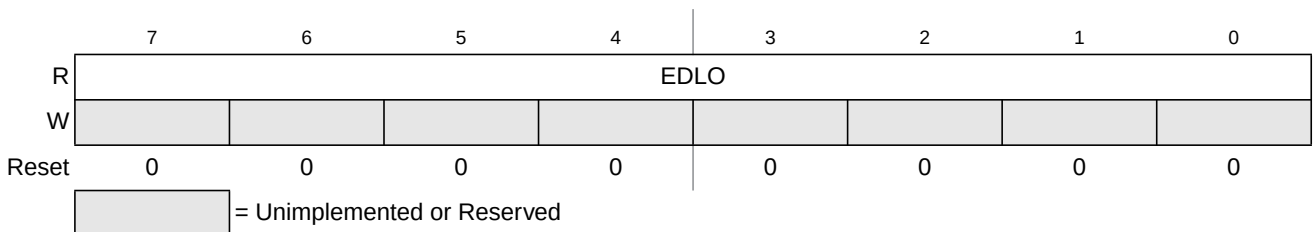
Figure 25-16. EEPROM Data Low Register (EDATALO)
