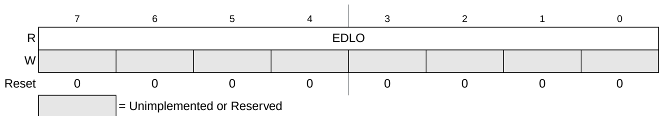
Figure 25-16. EEPROM Data Low Register (EDATALO)
