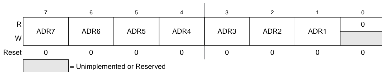
Figure 10-2. IIC Bus Address Register (IBAD)
