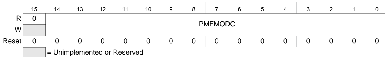
Figure 11-39. PMF Counter Modulo C Register (PMFMODC)
