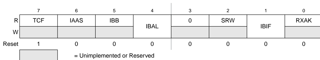
Figure 10-6. IIC Bus Status Register (IBSR)
