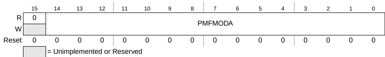
Figure 11-29. PMF Counter Modulo A Register (PMFMODA)
