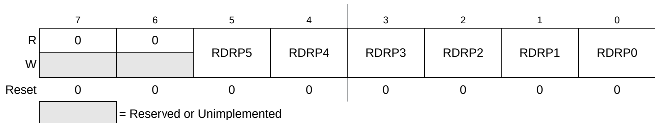
Figure 3-20. Port P Reduced Drive Register (RDRP)
