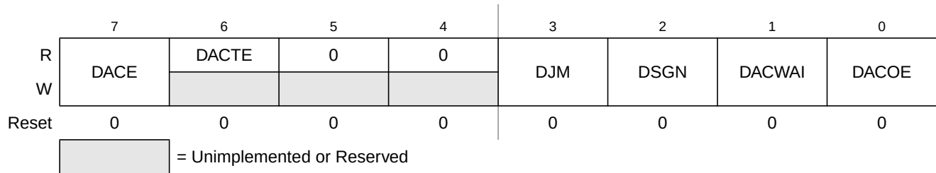
Figure 7-3. DAC Control Register 0 (DACC0)
