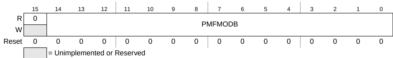
Figure 11-34. PMF Counter Modulo B Register (PMFMODB)
